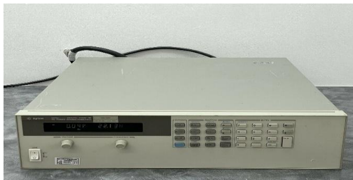
Figure 3. The AC power supply for electrical parameters measurements.
